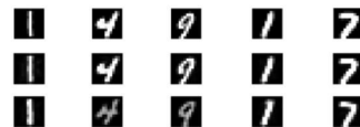
Fig. 1. Top: Original MNIST images downsampled to 12x12, Middle: Reconstructed images from bottleneck autoencoder, Bottom: D-Wave reconstruction from randomly selected imprinted features.
