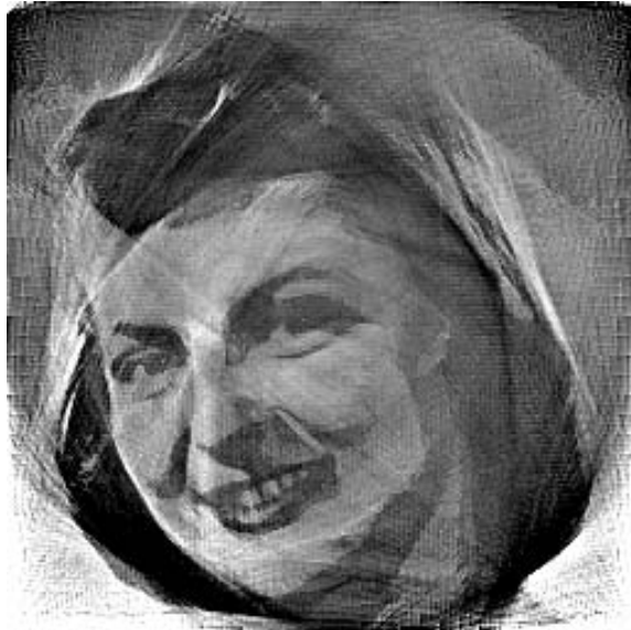
Figure 10: Result of taking the DMRT median transform of the test image S1 and then inverting it as if it were a DRT, not a DMRT. All of the detail shown is thus present in the median values of the original image along lines.
